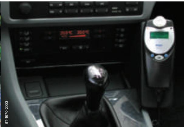
**Figure 2:** Dräger Interlock XT installed in a vehicle
